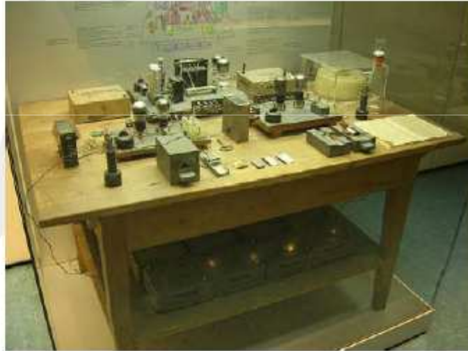
The experimental apparatus with which Otto Hahn and Fritz Strassmann discovered nuclear fission in 1938 © Wikipedia
